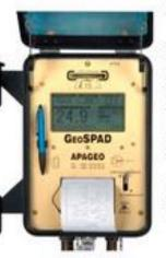
GEOSPAD<sup>M</sup> controls the conduct of Pressuremeter tests and automatically records the conditions and results of these tests.
